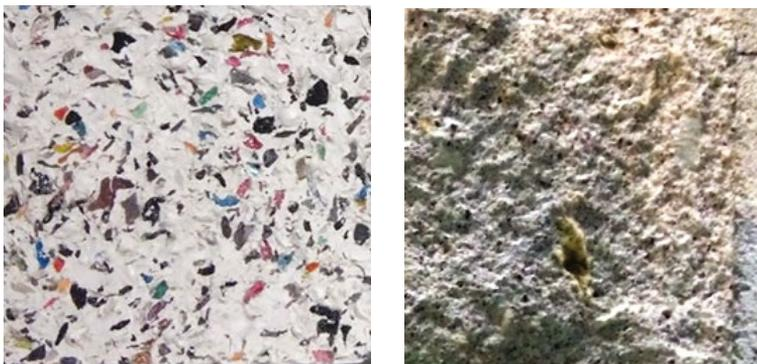
FIG. 5.2. Left: Plasterboard with plastic cable waste additives. Right: Cement mortar with mineral wool waste (Source: photos by A. Vidales Barriguete, 2020)
