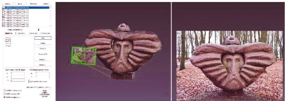
FIG. 2.3. Extraction of a real image model: orientation of sculpture “Bangpūtys” model, used 4 photographs (Source: own elaboration, 2020)
