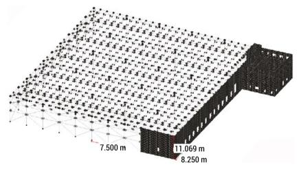
FIG. 8.3. Analytical model of wearhouse (Source: own elaboration, 2019)
