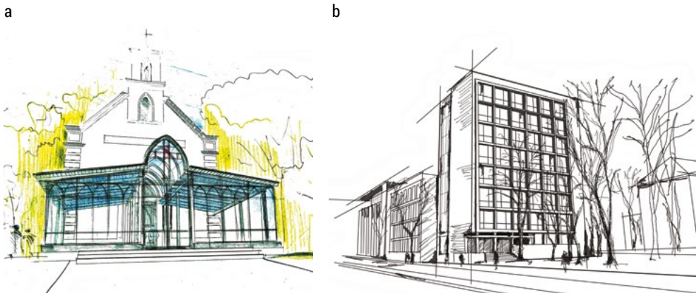
FIG. 2.8. Linear perspective projection – examples (Source: a – graphics by Marta Baum, b – graphics by Wojciech Matys)
